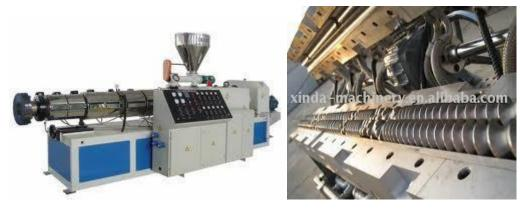
In twin-screw extruder, two screws are arranged side by side. One design incorporates screws they are intermeshing and self wiping. Since the screws rotate in the same direction, material moves helically along the inside barrel wall path from the feed section to the discharge point.
