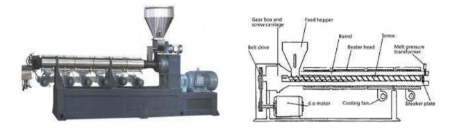
The heart of the extruder is screw. Its function is to convey resin blend from the hopper and deliver it into the die at a uniform rate and as a homogeneous melt. This blend is conveyed in three states: First, as a blend of solids (powder blend), then as a mixture of solids semifluxed crumb, and finally as a melt. To achieve these three basic types of fully flighted screw designs are in use,
