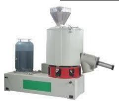
Generally, rigid dry blend will be processed with the high-powered intensive mixtures. Such blends must be dry, free-flowing powders with a minimum of agglomerates for extrusion of rigid pipe & profile extrusions. Dry blending should not be confused with preblending, which is just gentle physical mixing of ingredients. The main advantages of this compounding method are:
